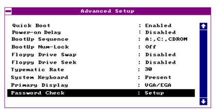
The first screen does not show all the parameters of the Advanced Configuration menu. To scroll down the rest of the parameters, press FGDN. Press 1 or 1 to highlight the desired parameter.
